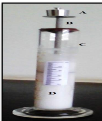
Figure 1 Gel strength measuring device (A)weights (B)device (C) graduated cylinder (D)gel Detachment Stress 5,6,7
