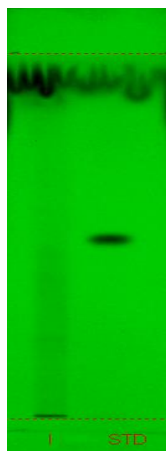
Figure 3: Alkaloid chromatogram before derivatization: Under day light, Under UV 366nm, and 254nm. Chromatogram after derivatization: under day light, Under UV 366nm.
