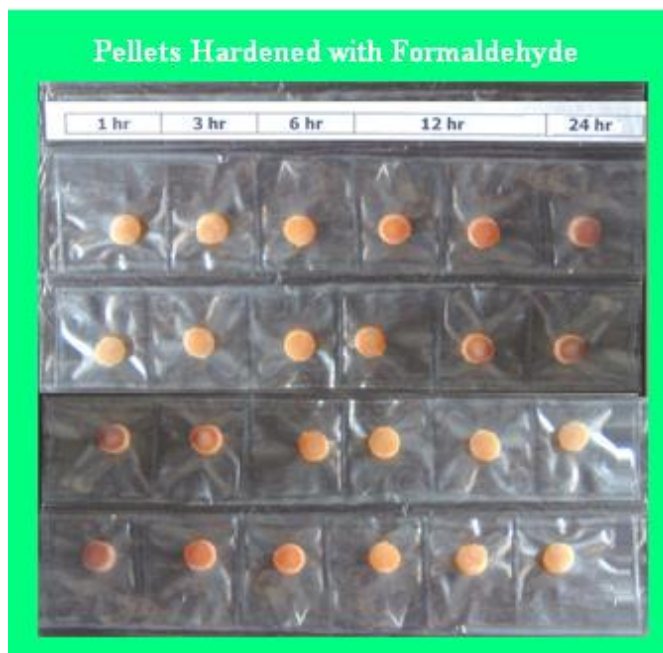
Figure 2: Pellets hardened with formaldehyde
