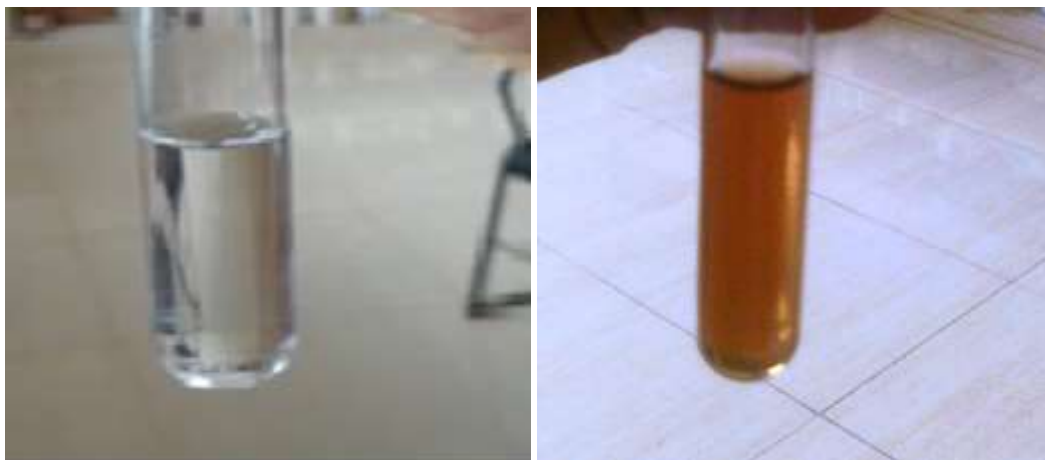
Figure 7: A) Image of Silver Nitrate solution B) Silver Nanoparticles produced using sodium citrate as reducing agent
