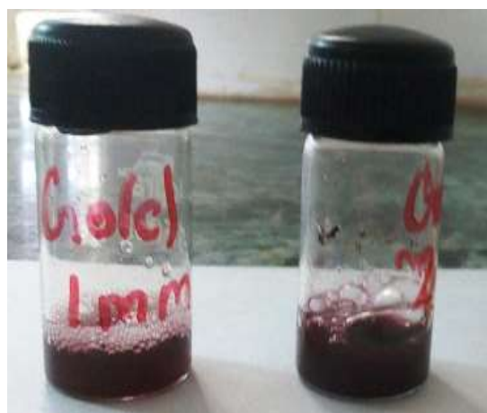
Figure 1: Appearance of purple color in solutions of 1mM and 2mM H 2 AuCl 4 indicating the synthesis of gold nanoparticles
