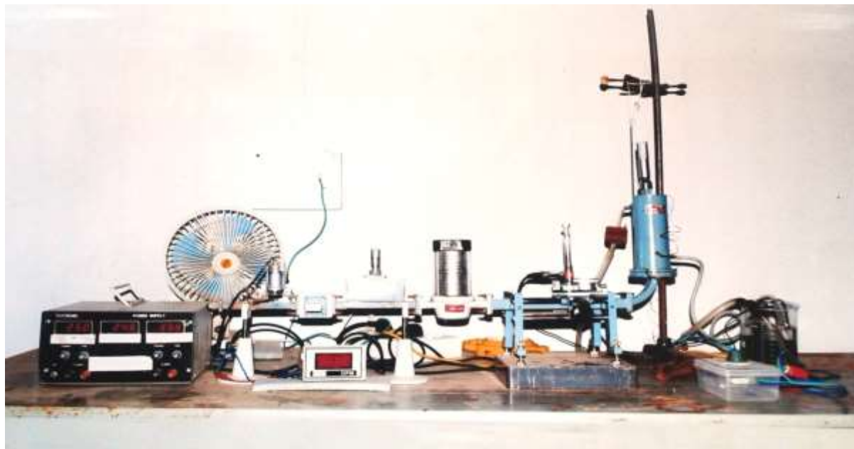
Figure 1: Experimental set-up for measuring dielectric constant and loss of a liquid, when sample length is in multiple of \lambda_d .
