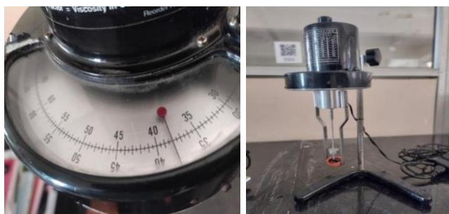
Figure 8: Measurement of viscosity using Brookfield viscometer
